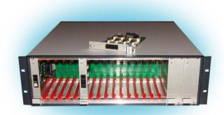
ASTEROID2-MT16 is designed for connection of the voice subscribers (lines) to IP PBX Asterisk/Freeswitch. The device allows connection of up to 128 phone ports FXS/FXO and up to 32 GSM ports. Connection to IP PBX is performed via the Ethernet network interface via the TDMoE protocol. Support of TDMoE in IP PBX is realized via the DAHDI program interface.
