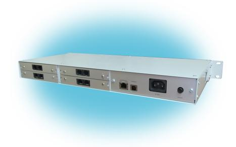
Asteroid-1U is designed for connection of telephone lines and GSM channels to Asterisk/Freeswitch. Server connection is made through Ethernet port using TDMoE protocol. The device is delivered as a chassis for 4 slots and a set of plug-in modules.
