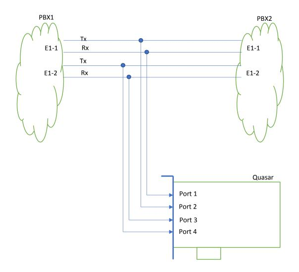
Since both E1 lines have their own signaling channel, two linkset sections need to be described. Scheme of connecting lines to ports RX1-TX1-RX2-TX2.
