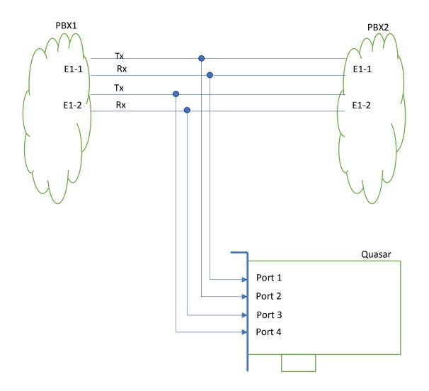
Both E1 lines share a common signaling channel (eg 16 on an E1-1 line), the group must be described in one linkset section. Scheme of connecting lines to ports RX1-TX1-RX2-TX2.
