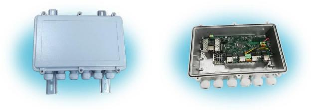
CR-603 is an Ethernet switch in a protected enclosure designed for operation in the industrial temperature range, with support for POE+ technology, support for SFP optical modules. The switch provides power and connects end devices to fiber optic lines at a speed of 1000 or 100 Mbps. The product provides power to external devices according to PoE 802.3at, 802.3af standards.
