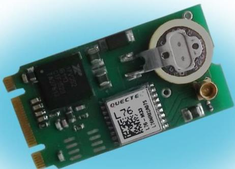
**The CR-508 module can be installed in fixed and mobile computers, onboard control units and controllers having an expansion slot M.2. The product provides the receipt of satellite navigation information from GPS and GLONASS systems and the transfer of navigational data to the computer - global coordinates, altitude, speed, exact time.**
