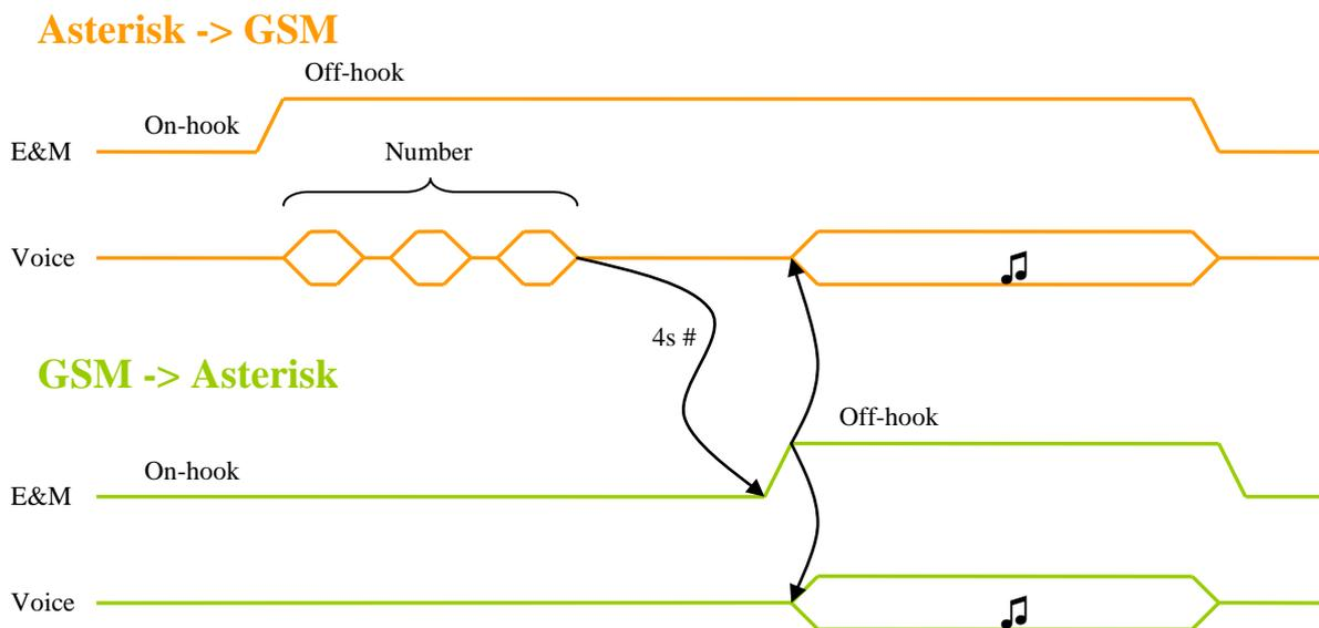
**Figure 8. GSM outgoing single call diagram**
