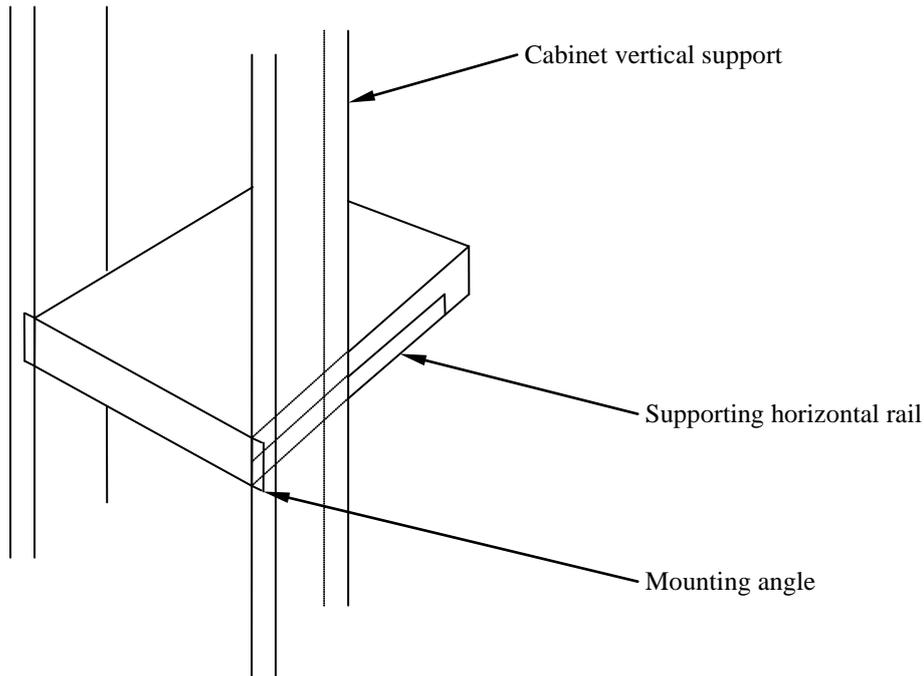
**Figure 3. Device assembly in a rack**
