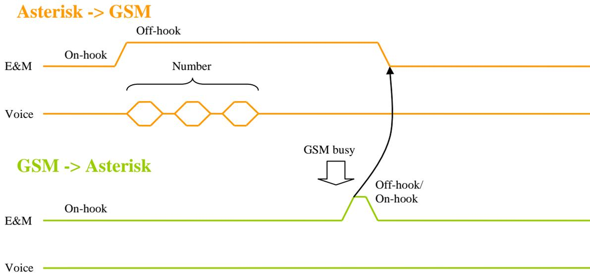
**Figure 10. GSM outgoing priority call diagram**
