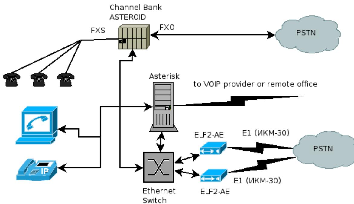
In this scheme the office can be connected to the IP telephony provider or corporate VOIP network. It allows to cut the expenses on telephony.
