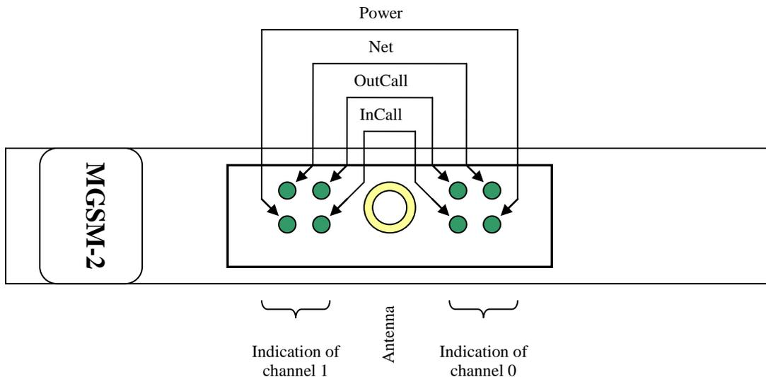
**Figure 6. Front panel of GSM module**
