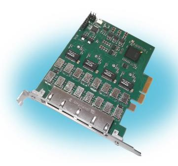
CR-701 is an adapter card in PCI-express format, designed for monitoring Ethernet networks 100 and 1000 base-T (twisted pair). The device provides interception of traffic from two external Ethernet lines, with the output of traffic to the PCI-Express bus of the hosting server.
