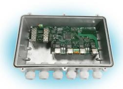
CR615 is a 7-port Ethernet switch in a rugged enclosure designed for operation in the industrial temperature range, with support for optical SFP and SFP+ modules. The switch provides connection of 5 ports according to the standards 1000 / 100base-T and 2 ports according to the standards 10Gbase-R/1000base-X.
