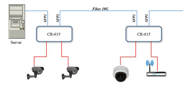
The switch allows you to connect external devices in both the point-to-point topology and the chain. Thus, coverage of an almost unlimited territory is achieved.
