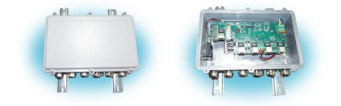
CR-613 is an 7 ports ethernet switch in a protected enclosure designed for operation in the industrial temperature range, with support for POE+ technology, support for SFP+ 10G optical modules. The switch provides connection of 5 ports according to the standards 1000 / 100base-T and 2 ports according to the standards 10Gbase-R / 1000base-X. On 4 ports the product provides power to external devices according to the standards POE 802.3at, 802.3af.
