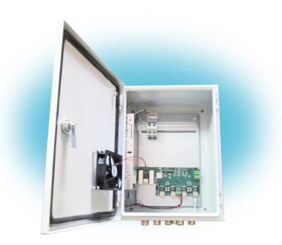
CR-610 is an 7 ports ethernet switch in a protected enclosure designed for operation in the industrial temperature range, with support for POE++ technology, support for SFP+ 10G optical modules. The switch provides connection of 5 ports according to the standards 1000 / 100base-T and 2 ports according to the standards 10Gbase-R / 1000base-X. On 4 ports the product provides power to external devices according to the standards POE 802.3at, 802.3af, 802.3bt.
