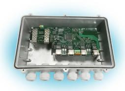
CR-605 is a 6-port Ethernet switch in a rugged enclosure designed for operation in the industrial temperature range, with support for optical SFP modules. The switch provides connection of 4 ports according to the standard 1000 / 100base-T and 2 ports according to the standard 100 baseFX / 1000base-X.
