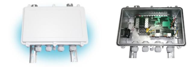
CR-602 is an Ethernet switch in a protected enclosure designed for operation in the industrial temperature range, with support for Ultra POE technology, support for SFP optical modules. The switch provides connection of the end devices according to the standard 1000/100base-T to fiber-optic lines with the speed of 1000 or 100 Mb/s. The product provides power to external devices according to PoE 802.3at, 802.3af or via a dedicated power connector.
