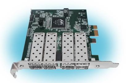
Adapter CR-509 designed as the combined device. Depending on configuration, it realizes one of three functions – multiport SFP GbE adapter, embedded switch in PC form factor or network tap.
