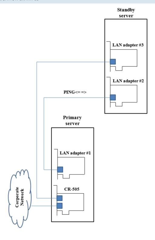
According to this scheme the primary server checks from time to time the connectivity to the standby server via LAN adapters #1 and #2. Adapter CR-505 is installed to the primary server and is connected to the standby server with a bypass port. If the connectivity is lost (or the software of
