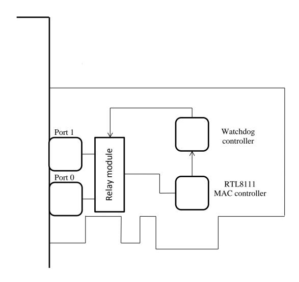
The device is based on MAC controller RTL8111, which port GBe is connected to the relay module. Depending on the mode, the relay module connects either the bypass port (port1) or the MAC controller to the main port (port 0). The relay module is operated with the help of the watchdog controller.
