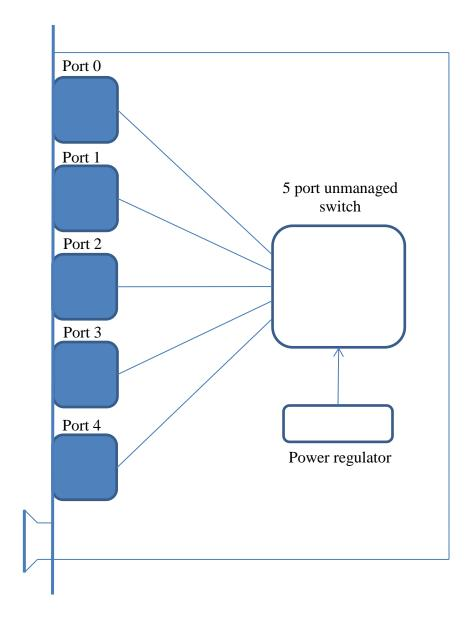
The device is based on 5-port switch RTL8367, which ports 0-4 are put to the front panel of the board.
