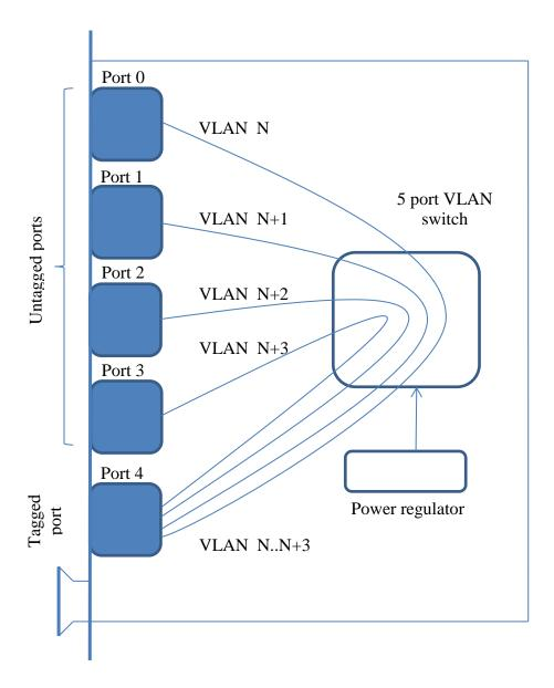
Tag N value is assigned by jumper configuration.
