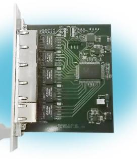
CR-503 is an Ethernet switch in the format of a 3U Eurocard (according to the mechanical standards of IEEE 1101.1 and IEEE 1101.11). The device has 5 Gigabit Ethernet ports and can be used in several modes: as an unmanaged general-purpose switch, as a switch with VLAN functions, or an Ethernet tap. The board format allows installing the device to the expansion slots of crates CompactPCI, PXI, VME, VME64 and other bus-structured modular systems complying with IEEE 1101.1 standard.
