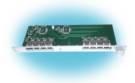
CR-502 is an Ethernet switch in the format of a 6U Eurocard (according to the mechanical standards of IEEE 1101.1 and IEEE 1101.11). The device has 8 Gigabit Ethernet ports and can be used in several modes: as an unmanaged general-purpose switch, as a switch with VLAN functions, or an Ethernet tap. The board format allows installing the device to the expansion slots of crates CompactPCI, PXI, VME, VME64 and other bus-structured modular systems complying with IEEE 1101.1 standard.
