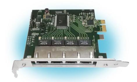
Adapter CR-501 designed as the combined device. Depending on configuration, it realizes one of three functions – multiport Ethernet adapter, embedded switch in PC form factor or network tap.
