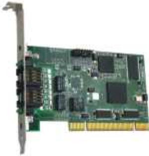
QUASAR-mini E1 PCI adapter for IP PBX Asterisk/CallWeaver
