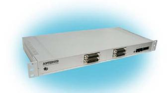
Asteroid can be used for attaching up to 30 telephone lines to the traditional PBX or to the Asterisk/CallWeaver. It can be connected to the traditional PBX with the help of E1 interface. Connection with Asterisk can be made through Ethernet port, using TDMoE protocol.
